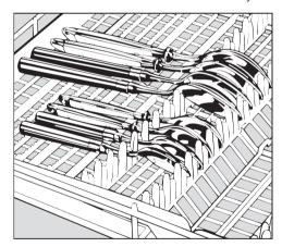
If spoon handles do not fit between the holders then lay them the other way round making sure that the head of the spoon is in contact with the support on the bottom of the tray.
